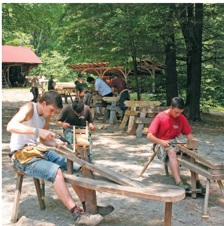
At left, French apprentices directed by Heartwood School student Ben Theriault (at right in bandanna) lay out rafters in Washington, Mass. At top, Martin Lorentz, seated at the Millers Falls boring machine, and Boris Noël, standing at right, compagnons who came from Troyes to help supervise the 20 French apprentices (or rabbits). Above, apprentices intently shaving pegs split out from block.
